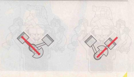
TWO-TIMER Adding a piston at a 90-degree angle (creating a 90-degree V-2) allows the counterweight to balance both pistons throughout their travel. The counterweight cancels the up-and-down motion of one piston, and 90-degrees later, cancels the motion of the other piston. Unlike the singlecylinder example, the counterweight is balanced throughout its motion.
