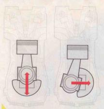
PART-TIMER In a one-cylinder engine, the up-and-down motion can be balanced by the counterweight. When the piston is at the top of its travel (shown), or the bottom, the counterweight offsets the mass of the piston. But when the piston is not at the top or bottom of its travel, the weight induces a left/right imbalance.
