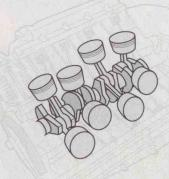
EIGHT IS ENOUGH A 90-degree, cross-plane V-8 is essentially a collection of four 90-degree V-2s (see V-2 illustration on previous page). Since each V-2 is balanced, the cross-plane, 90-degree V-8 also is free of rotational and reciprocating motions. Firing forces are balanced because they occur at every 90-degree turn of the crank.
