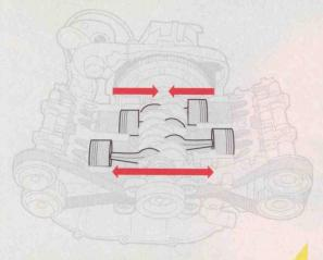
BOXER BASICS In a flat (180-degree) engine, each bank of cylinders exactly mirrors the other and, consequently, the forces are canceled and the engine's up-anddown and rotational forces are balanced. The firing forces are also balanced as firing events take place every 180 degrees.
